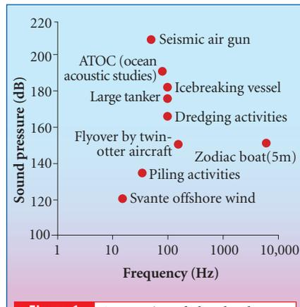
**Figure 1** A comparison of selected underwater anthropogenic noise sources (peak intensities taken from Richardson et al., 1995 and Westerberg, 1999)
